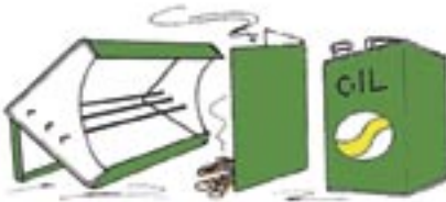
Reflector stoves made from oil drums and cans or sheet metal
