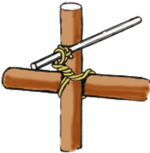
Tourniquet lashing (tightening the lashing)
